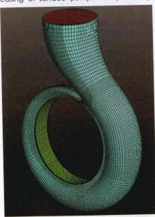
The geometries are transformed in mathematical models: This way, even before the testing room phase, flow head and absorbed power data are available. The mathematical model can be modified in order to improve the performances in percentage points and to decrease the absorbed power. Moreover, SAER has the possibility to test the projected parts even before the casting, through the prototype machine. All the trials on the pumps and motors are made in the two internal mod-
